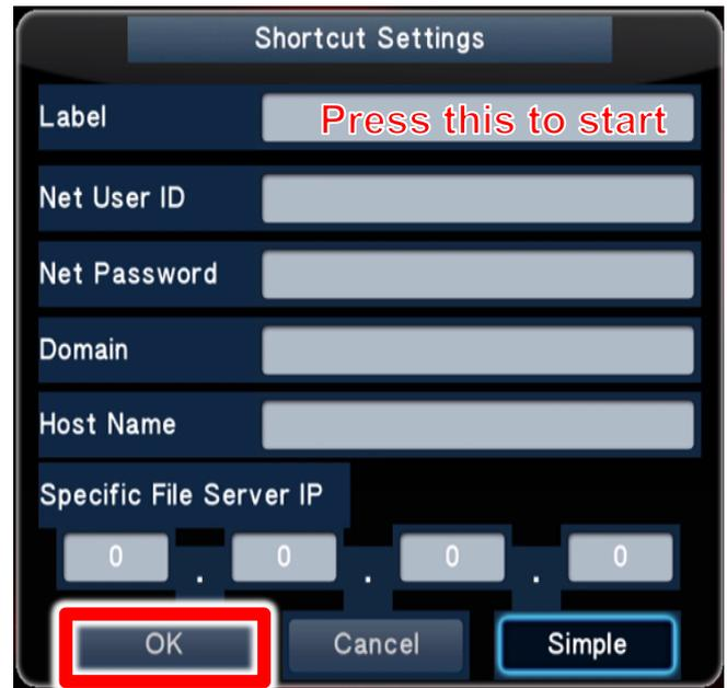
Enter the user ID (please enter the account of player box, for example, the first one is client1, others reference FL operation manual), network code, specific file server IP (The preset of FL is 192.168.1.170) in order. After entering, choose “detail” and set the label name as Press “OK” button, and then press Enter.
