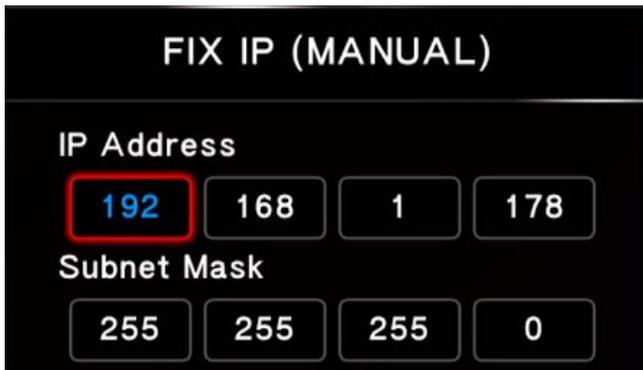
In the FIX IP(manual) window, the subnet mask is set as 255.255.255.0
