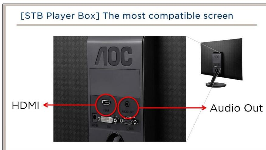
Device connection diagram as below. Attention that the earphone is connected to the monitor audio output (Audio Out). Earbuds is 3.5mm interfaces.
