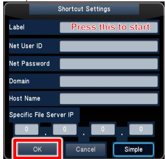
Enter the user ID (please enter the account of STB player, for example, the first one is client1, others reference factory preset list), network code, specific file server IP (The preset of SES is 192.168.1.169) in order. After entering, choose “detail” and set the label name as Press “OK” button, and then press Enter.
